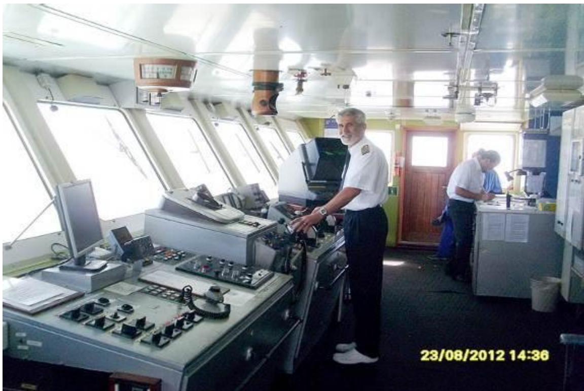
Command bridge of m/v »Larkspur« used for chart positioning
